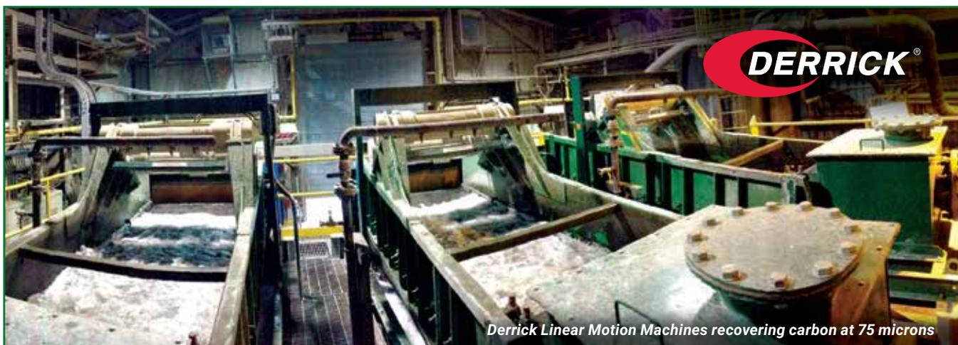
Derrick Linear Motion Machines recovering carbon at 75 microns
