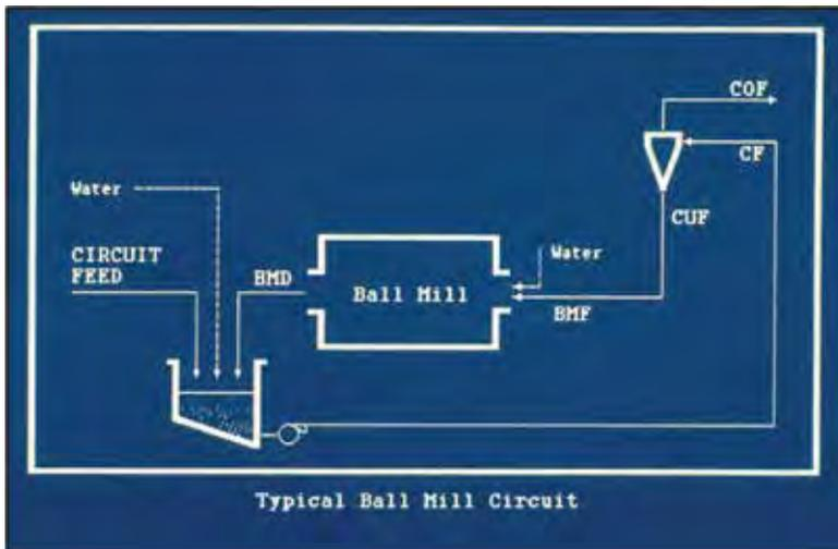
mill feed and discharge size distributions using a first-order rate equation. By calculating these cumulative grinding rates for all screen sizes, a complete ball mill model is generated (as used by Finch and Ramirez, 1981). Others in industry, Hinde and Kalala (2009), for example, have noted the same. Lacking the complexity needed to maintain their interest, most researchers have ignored this model, broadly
